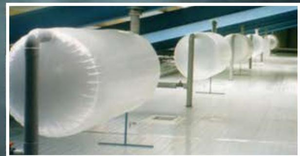
All our CO<sub>2</sub> Adsorbers are equipped with low oxygen lungs / buffers. This is important to achieve extremely low oxygen percentages and enable ACR. A low oxygen lung also contributes to energy efficiency, because no N<sub>2</sub> needs to be added by a generator
