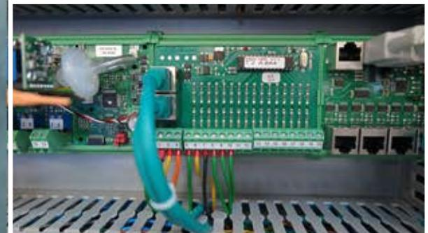
Standard provided with alarm contacts for compressed air, thermal and over voltage. This improves the reliability of the system so that the machine remains low in maintenance
