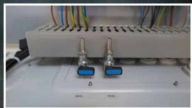
All our adsorbers are equipped with an adsorption and regeneration tap. This allows a service technician or yourself to easily measure the capacity and leak-tightness of the system
