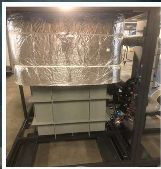
Insulated Catalyst bed and heat exchanger in one
