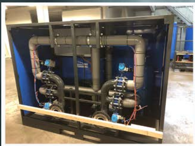
4 pneumatic valves incl. open/close indicator
