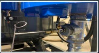
The carbon filters are equipped with pollution oil indicators. if the white powder inside the oil indicator becomes yellow due to compressor oil it means the carbon filter has to be changed. This way we guarantee maximum protection of the lifespan and capacity of the CMS.
