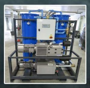
The oil-free blower used in our VPSAs ensures that the active carbon is not contaminated by residual oil in combination with low pressure. resulting in its life-expectancy more than doubling. Life span carbon (CMS) > 10 years.
