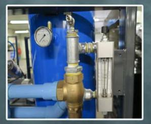
The flow indicator on the outlet side has a valve to manually adjust the flow You can read the flow by the level of the floater in the transparent tube. You can connect measuring equipment to the tap to measure and check the purity.
